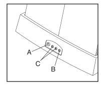
To connect an external device such as a VCR, use the jacks labeled C. To use an external device, you will need to select the Line In mode. To select the Line In mode, press and hold down the Play and Volume increase buttons simultaneously for about five seconds. The indicator above the lonizer button will flash.
